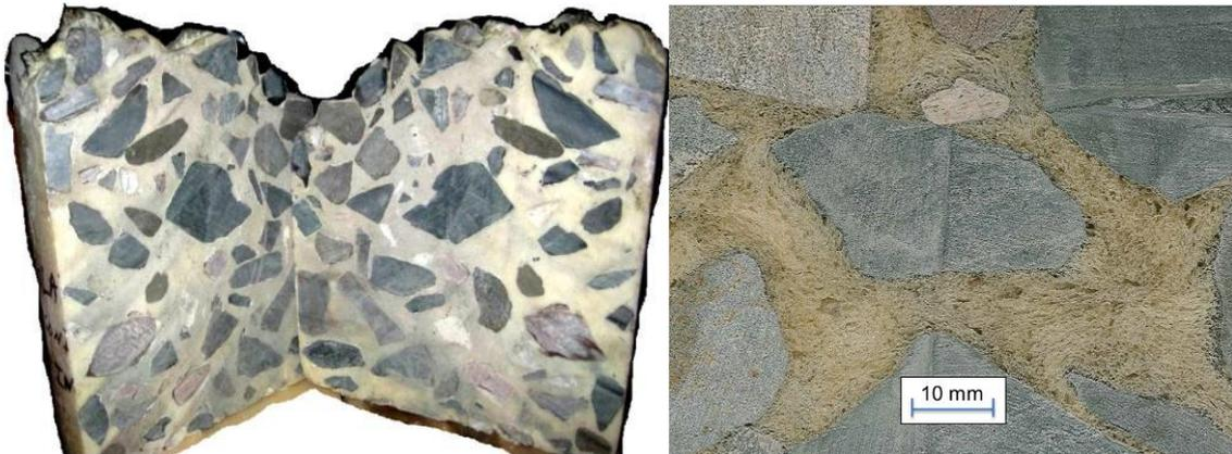
Figure 1: A PSB specimen cut in half using a concrete masonry saw shows the complete void filling by the expanding foam (left) and a close-up photo is shown (right).
